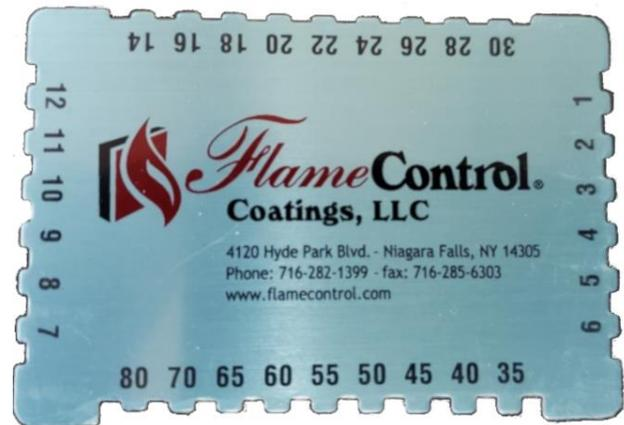
A wet film gauge like the one above can be utilized to determine the mil thickness of the paint film that has just been applied.
